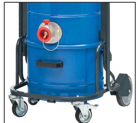
The air flow is diverted to clean the filter.
