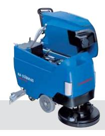
Fresh water can be filled up in an instant – via the integrated, industry-standard system connector or via the large filling opening.
