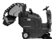
Hydraulic high-dumping system 21 132 430Z
