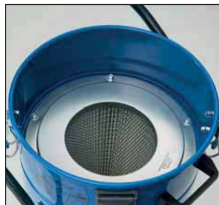
Filter cartridge with 30,000 cm 2 filter surface area
