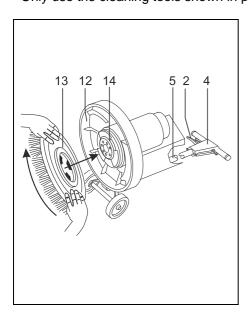
Only install the cleaning tool by hand.
