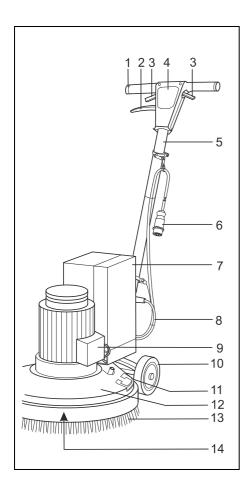
The cleaning tool (13), should always be removed from the appliance. Release the wheel assembly by pressing the pedal between the wheels. Tilt the machine backwards so that the control unit (4) rests on the floor.
