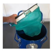
Loose the clamp and remove the remove the polypropylene filter for vacuuming liquids. Fit the new filter and tighten with the clamp. Fit the entire assembly in the container. Fit the float and motor head and secure with the two safety retainers.
