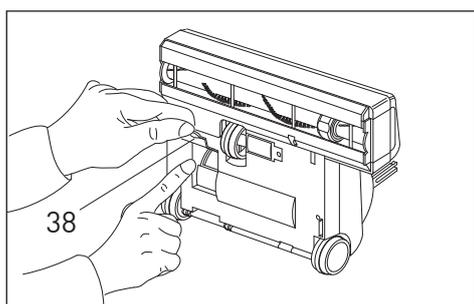
If the hose and tube are clear, check the swivel neck (20) by looking down the neck where the tube fits. Also check the trap door (38) underneath the machine. Ensure the passage between the trap door and the exit to the tube is clear.
