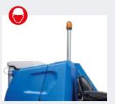
**SECURITY KIT**Rotating beacon for maximum safety during operation
