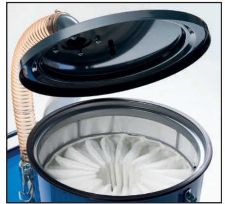
Filter cartridge with 30,000 cm 2 filter surface area
